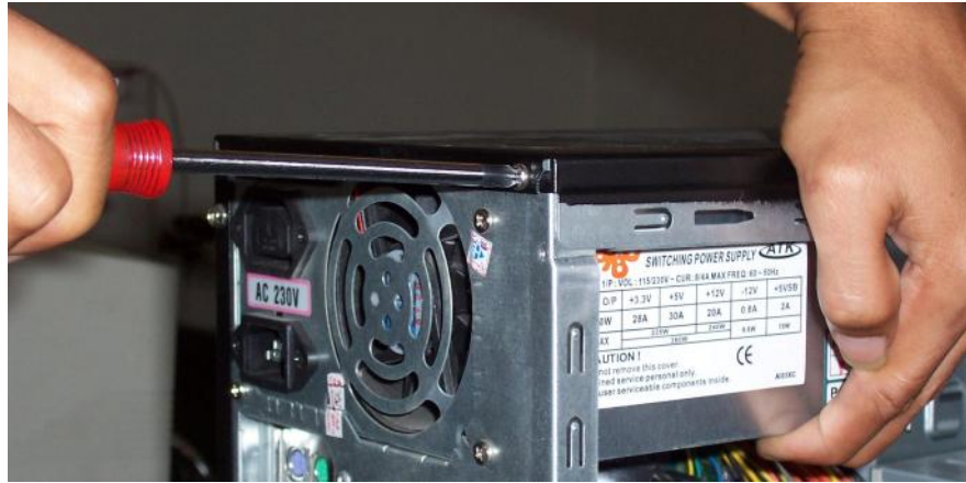
Gambar 3. 4. Memasang Power Supply
